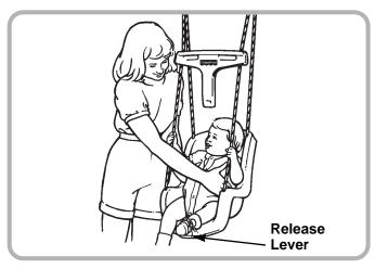
The release lever is located on the underside of the swing seat. Squeeze the release lever toward the front edge of the swing and lift the restraint bar. Slide the restraint bar up.
